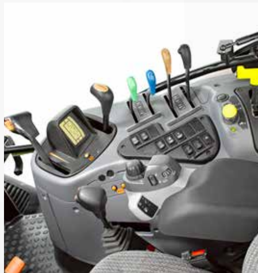
Profi Classic equipped with mechanical control units and electronic hitch control (EHR).
