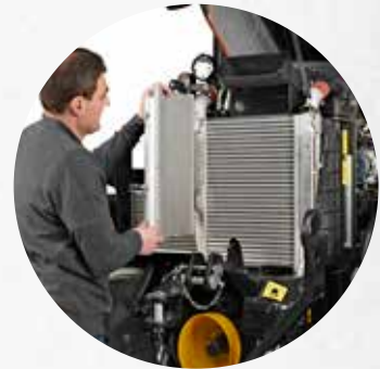
Fast and simple cleaning of the radiator and air-conditioning system.
